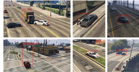
Fig. 6. Some examples of correct anomaly detection, when the trained Faster R-CNN is executed on synthetic test videos. From the top-right, clockwise: traffic collision , vehicle on pedestrian area , car in wrong way , risky overtaking , car in no parking area and red light violation .
